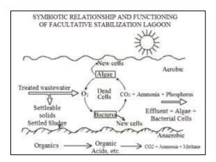
Figure 5 Facultative Lagoon Treatment of Sludge<sup>13</sup>
